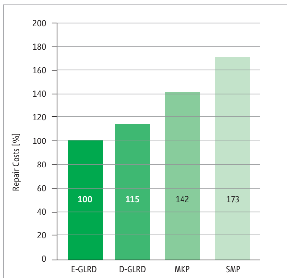
Figure 6: Maintenance costs of various types of centrifugal pumps
